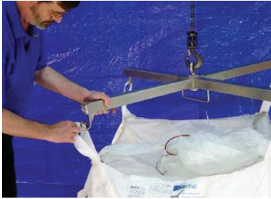
Attaching the restraint to lifting bar
