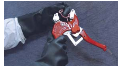
Load crimp into installation tool
