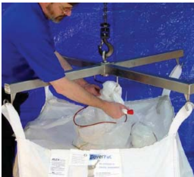
Securing the liner neck
