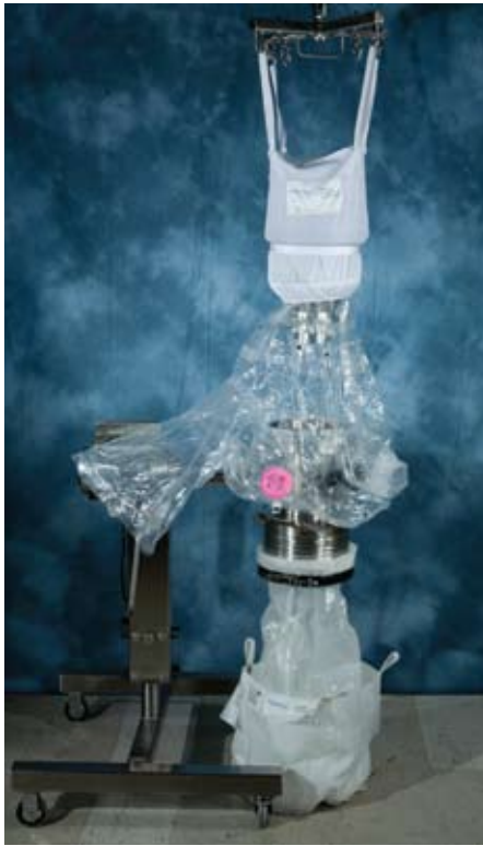
Figure 2. Shroud used to hoist canister.
