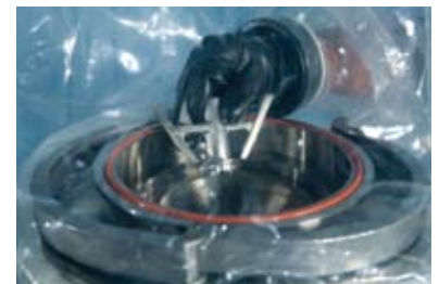
Figure 4. Integral glove sleeve for manipulating screen.
