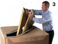
3. While holding on to the filling fitment, carefully lower the cassetted liner into the IBC, taking care that the dispense fitment will be aligned on the correct sidewall of the IBC once the cassette is fully opened.
