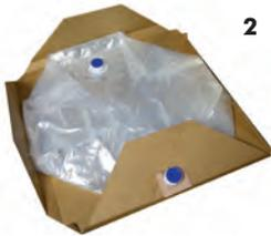
2. Open the cassetted liner package and remove the protective wrap on both the fill and dispense fitments. Remove the locking ring and place aside for use later. Remove the protective cap from the dispense fitment. Fully extend, and even hyper extend, the flap on the cassette where the dispense fitment is secured. (this will help in positioning the dispense fitment with the dispense port on the IBC body)
