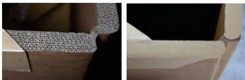
Also for additional security, the corrugated flutes of the container are covered to insure that the container is hygienic and contaminant free.
