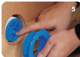
5. The dispense fitment should be accessible through the dispense port. Reach through the dispense port and, with your fingers inside the fitment, pull the dispense fitment snugly into the port. Insert the locking ring into the port and begin threading the ring onto the dispense fitment. Finish tightening the ring with the locking ring tightening tool and thread the protective cap back onto the dispense fitment.
