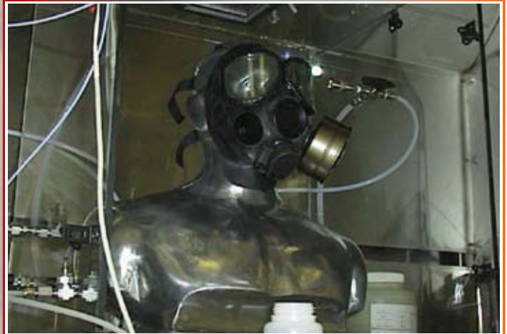
Simulant Agent Resistant Test Manikin (SMARTMAN) Headform shown with M40 mask .
