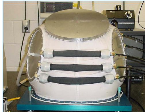
Figure 9. Fluidic Muscles Installed on X-Large SUT
