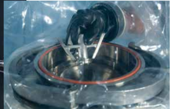
Mill impeller and screen change out
