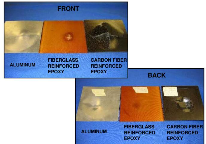
Figure 8: Results of Impact Testing at 300 ft-lbs
