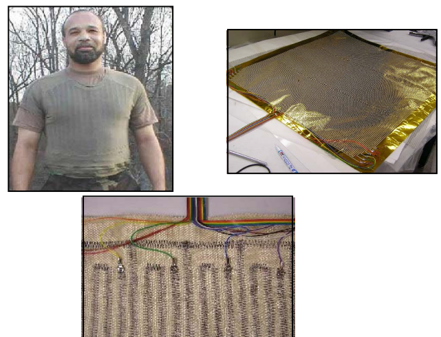
Figure 12. Sensate Liner, Traces on Film and Fabric
