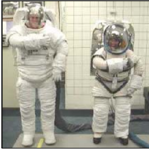
Figure 7. Small Size Waist Entry I-Suit and Large Size Shuttle EMU
